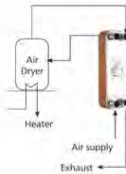
Hot circulation dryer circuit
